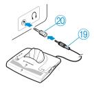
▶ Plug the other end of the connection cable (9) into the head-phone socket on your sound source.
